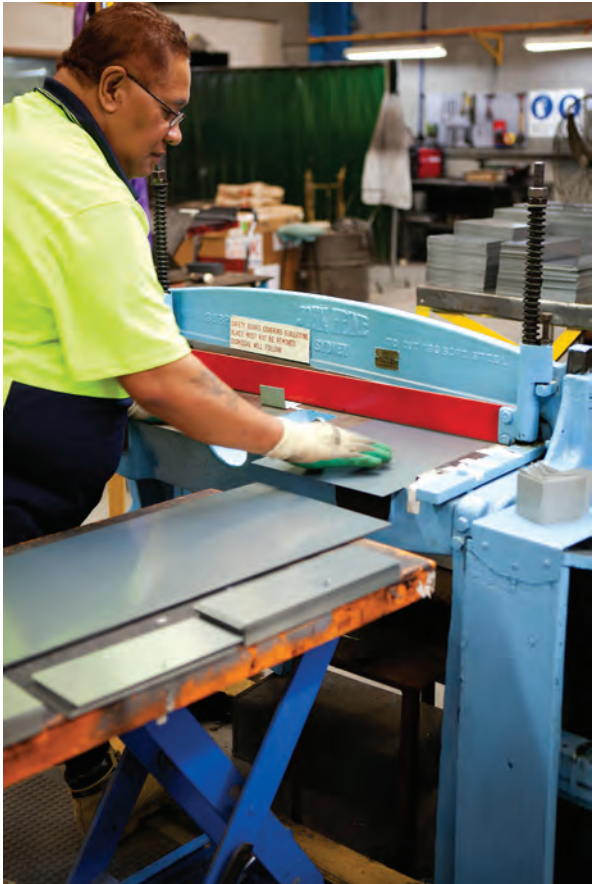
Cutting core strips and yokes
