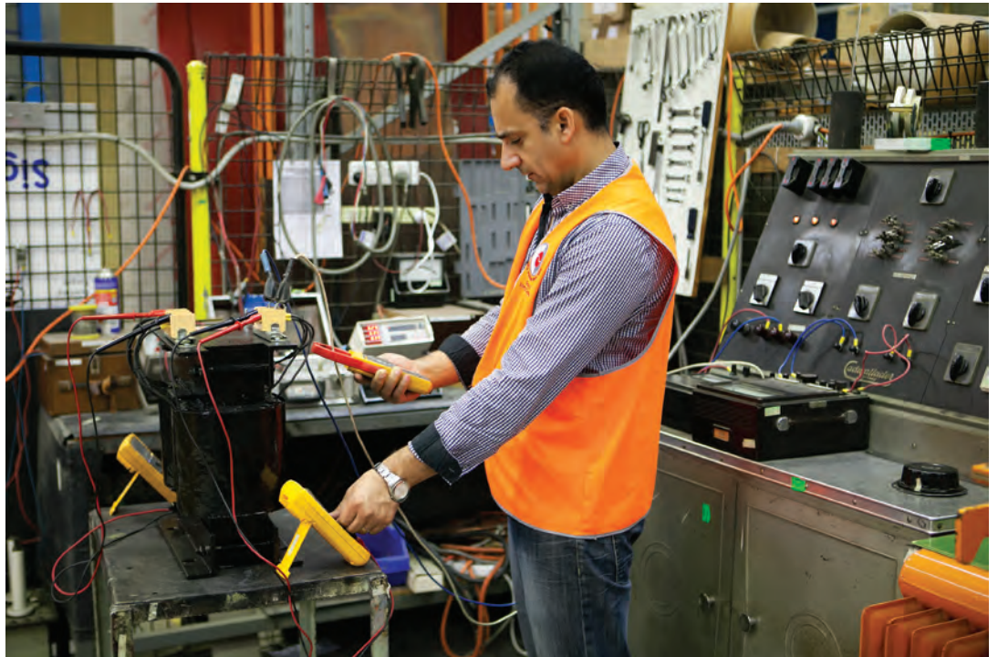
Testing of Single Phase Power Transformer
